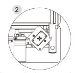
Insert the hexagonal post of the lifting column into the corresponding hole in the desktop.
