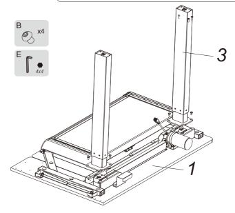
Connect lifting columns (3) to the desktop (1) using screws (B) and wrench (D).
