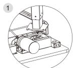
Insert the hexagonal post of the lifting column into the corresponding hole in the desktop.
