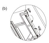
After the extension board is installed, you can adjust the angle of the support rod according to your own needs (as shown in Figure a) so that the extension board assembly can be expanded. If not needed, collapse the extension rods as in Figure b.
