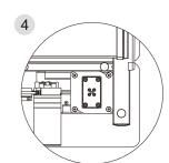
Use 4x4 wrench (E) to tighten down screws (B).
